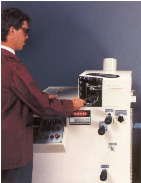
Operator inserts drill to be ground into the Workhead. There is no need to manually hold the drill during the grind cycle.
